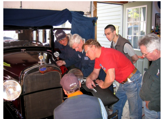
The headlight station checks the focus and alignment in the darkened garage. Proper adjustment makes a huge difference. We have had to fix all kinds of electrical problems.
