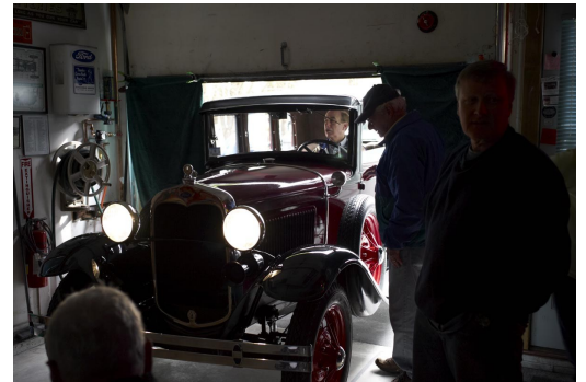
The headlight station checks the focus and alignment in the darkened garage. Proper adjustment makes a huge difference. We have had to fix all kinds of electrical problems.
