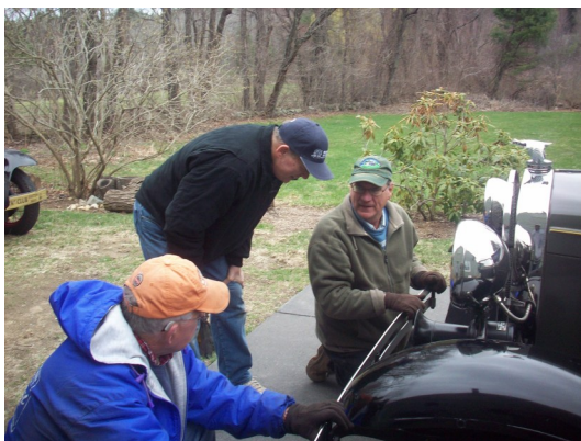
Above: Toe-in being checked using the Ford approved gauge. Below: Clutch free play checked
