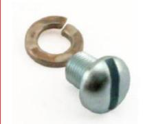
The problem is that the ignition cam screw may not hold the cam down tightly to the distributor shaft. After a bit of driving, the cam rotates into a more and more "retarded" position and the engine loses power.
