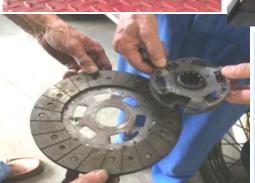
As you can see the clutch was totally destroyed. A clutch spring got dislodged and caused the three rivets to be ripped out of the of the center portion of the clutch. A new disk and pressure plate solved the problem.
