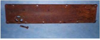
Get all of the screws started, and then go around and tighten them all up in several passes. Have the screw head just touching the piece at first, then make them all snug, then make them all fully tightened. Just like you do when tightening head nuts, start with tightening the screws in the middle and then work your way out to the ends. Alternate sides left and right as you go on each tightening pass.
