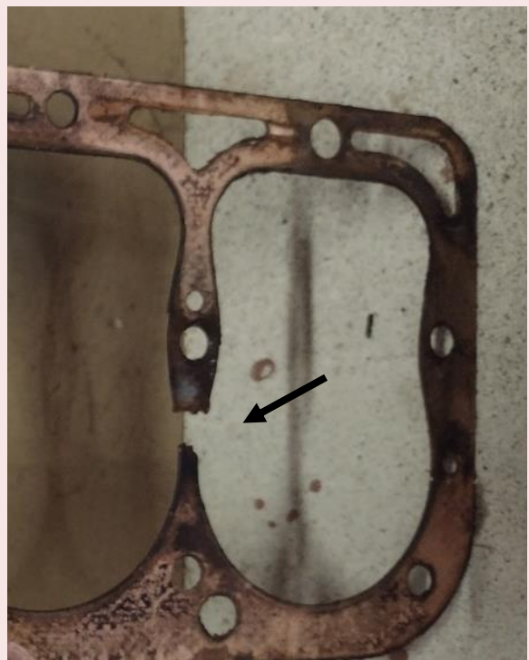
The break in the head gasket
